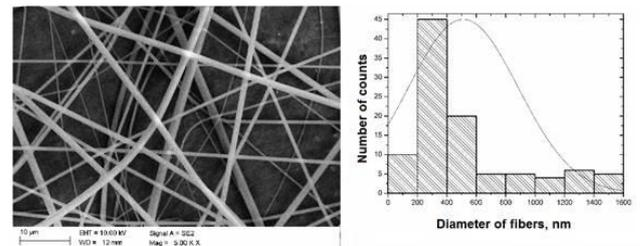
Fig. 3. The SEM image of the obtained PVP nanofibers for sample no 2 and histogram showing the values of nanofibers diameters
