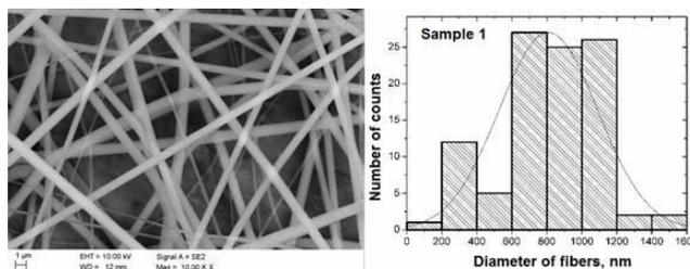
Fig. 2. The SEM image of the obtained PVP nanofibers for sample no 1 and histogram showing the values of nanofibers diameters
