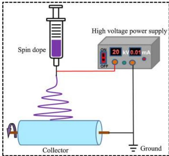
Fig. 1. Schematic illustration of an electrospinning process [18]
