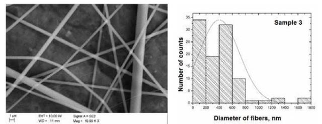
Fig. 4. The SEM image of the obtained PVP nanofibers for sample no 3 and histogram showing the values of nanofibers diameters
