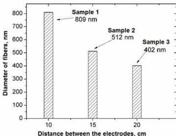
**Fig. 5.** Histogram showing the average nanofiber diameters for the obtained fibrous mats with various distance between the electrodes
