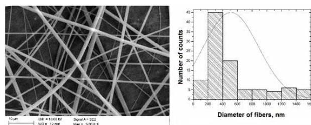
Fig. 3. The SEM image of the obtained PVP nanofibers for sample no 2 and histogram showing the values of nanofibers diameters
