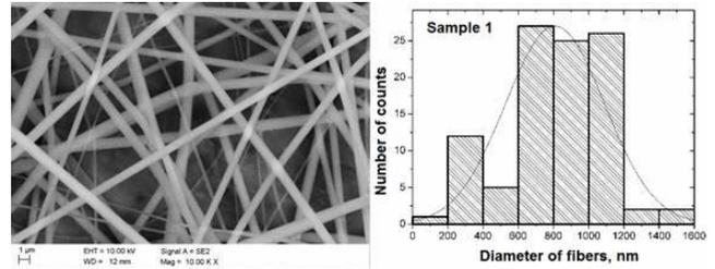
Fig. 2. The SEM image of the obtained PVP nanofibers for sample no 1 and histogram showing the values of nanofibers diameters
