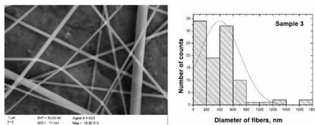
Fig. 4. The SEM image of the obtained PVP nanofibers for sample no 3 and histogram showing the values of nanofibers diameters
