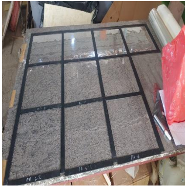
Fig. 4. Open Mold Setup at M/s. Vaishnav Composites
