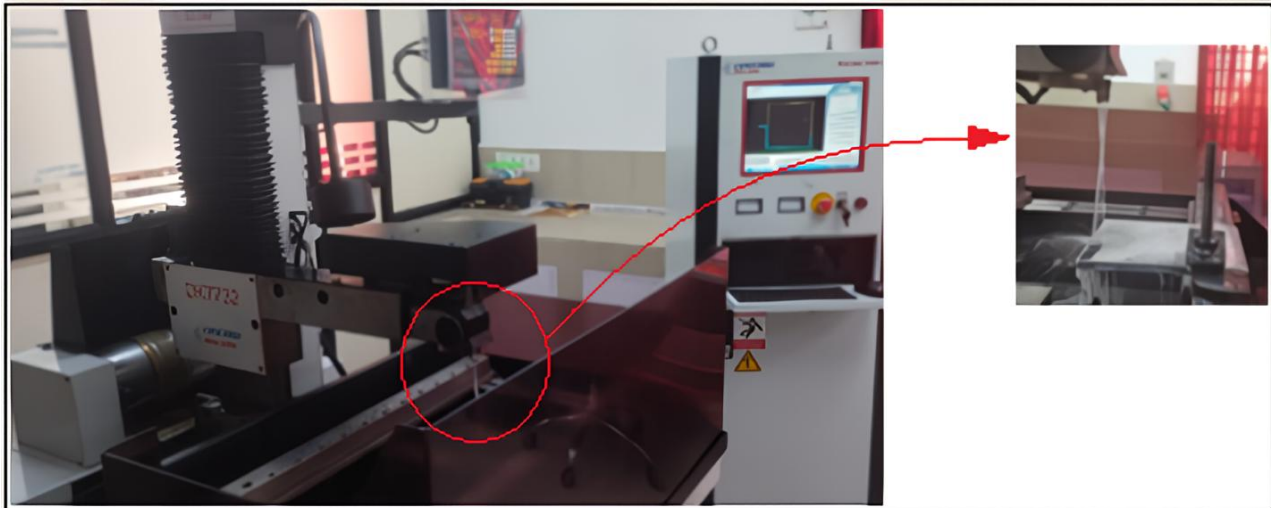
Fig. 1. Workpiece fitted with the WEDM experimental setup [16]
